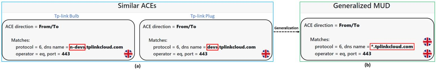
Figure 4: MUDs Comparison (a) and generalization (b) of two different devices of the same manufacturer
