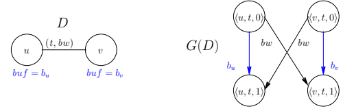
Fig. 2. Example of constructing event-driven graph G(D) from a delay-tolerant network D with a single contact.
